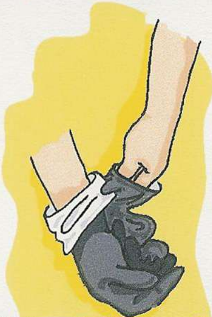
3 With the cuff of the removed glove nip the cuff of the second glove
